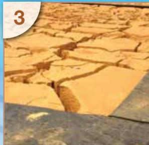
At a neutral pH, the iron can no longer stay in solution and precipitates out as iron oxide suitable for use as a pigment. When enough material is collected, it is harvested.
